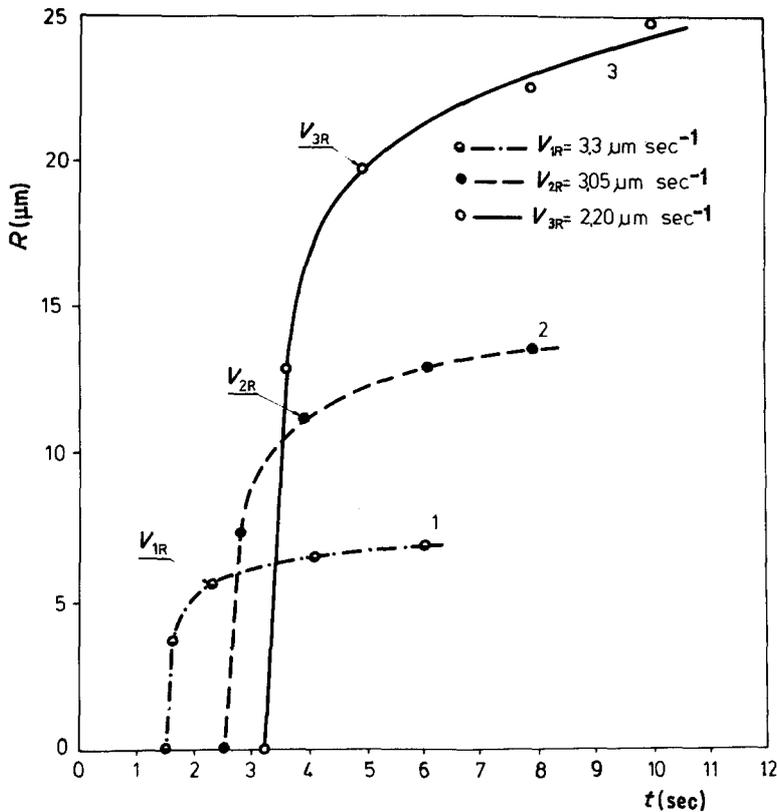
Figure 6 Dependence of dendrite radius  $R$  on time of solidification time of Al-40 wt % Zn alloy.
