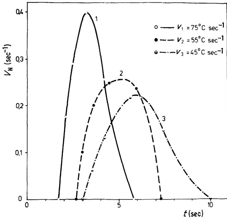
Figure 7 Changes of volumetric growth rate  $V_N$  against solidification time of Al-40 wt % Zn alloy freezing at: curve 1, 75 K sec<sup>-1</sup>; curve 2, 55 K sec<sup>-1</sup>; curve 3, 45 K sec<sup>-1</sup>.
