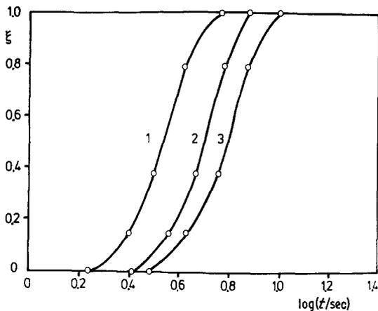
Figure 3 Kinetics curves of solidification of Al-40 wt% Zn alloy.
