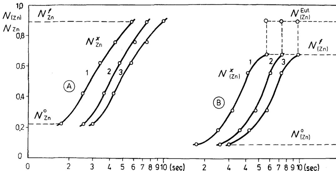
Figure 2 Changes in the zinc concentration during solidification of Al-40 wt% Zn alloy, cooled at the following rates: curve 1, 75 K sec<sup>-1</sup>; curve 2, 55 K sec<sup>-1</sup>; curve 3, 45 K sec<sup>-1</sup>. (A) mole fraction of zinc in liquid ( $N_{Zn}^l$ ); (B) mole fraction of zinc in a dendrite  $N_{(Zn)}^x$ .
