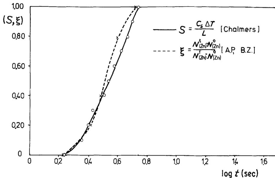
Figure 8 Kinetic curves of solidification given by Chalmers [17] and the authors.  $S$  is the fraction of solidified phase;  $T$  is the supercooling;  $L$  is the latent melting heat.
