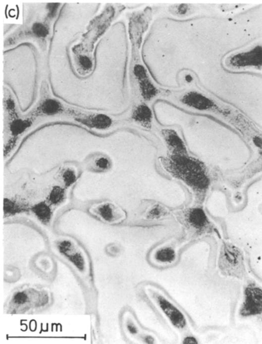
Figure 5 Dendritic microstructures of Al-40 wt% Zn alloy solidifying at rates: (a) 75 K sec<sup>-1</sup>, (b) 55 K sec<sup>-1</sup>, (c) 45 K sec<sup>-1</sup>.
