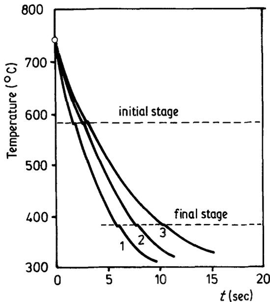
Figure 1 Cooling curves of Al-40 wt% Zn alloy solidified at different rates: curve 1, 75 K sec<sup>-1</sup>; curve 2, 55 K sec<sup>-1</sup>; curve 3, 45 K sec<sup>-1</sup>.
