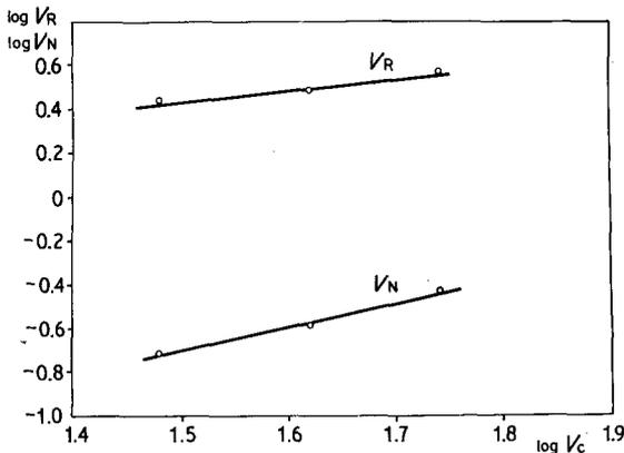
Figure 9 Plot of linear solidification growth rate  $V_R$  and volumetric growth rate  $V_N$  against the cooling rate  $V_C$ .
