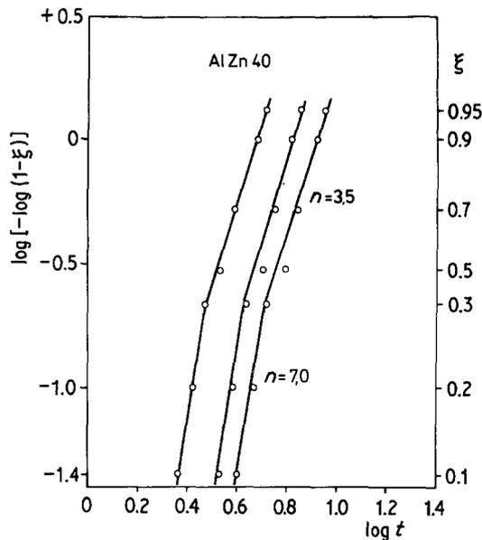
Figure 4 Analysis of the solidification kinetics of Al-40 wt% Zn alloy on the basis of Johnson-Mehl equation.
